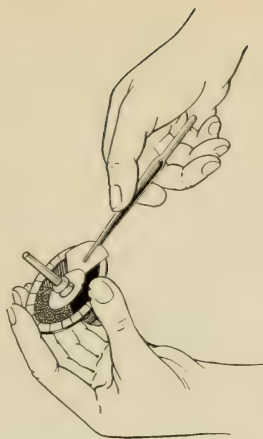
Fig. 3. The Color Top and Method of adjusting the Color Disks.
